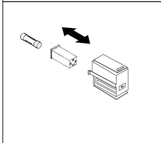
**3** Rotate line voltage selector and reinstall so correct voltage appears in fuse holder window.
