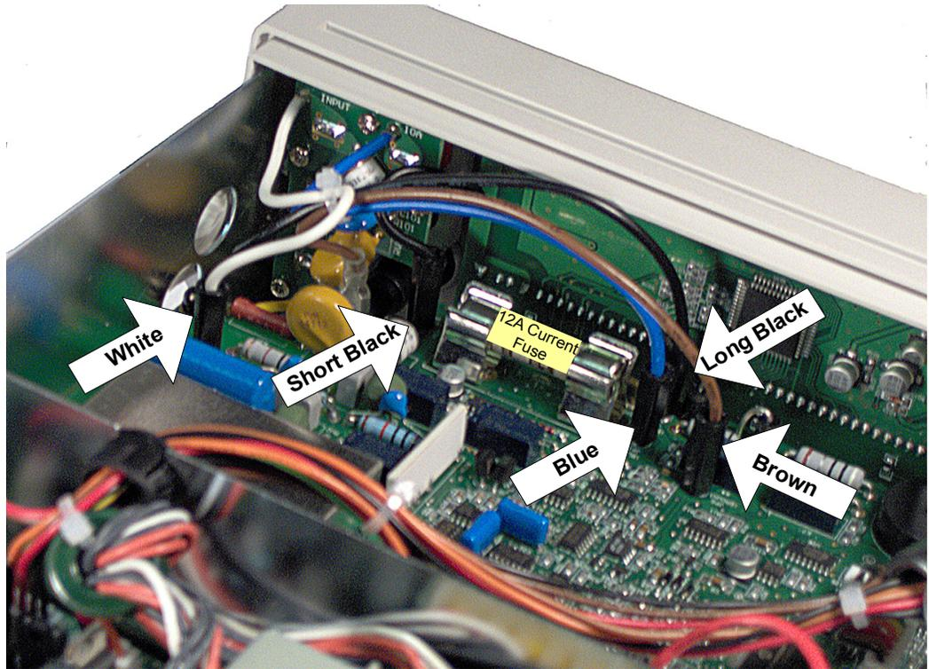
10 There is now enough play to allow the side of the front panel to be pried from the chassis and removed as an assembly.
