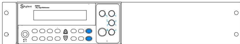
To rack mount two instruments side-by-side, order lock-link kit 5061-9694 and flange kit 5063-9212.
