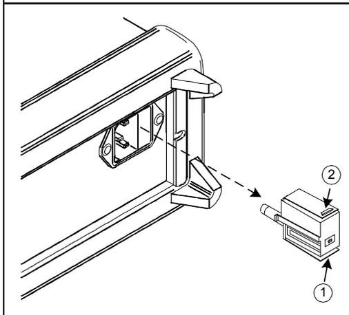
**2** Remove the line voltage selector from fuse holder assembly.
