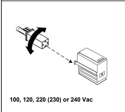
**4** Replace fuse holder assembly in rear panel.
