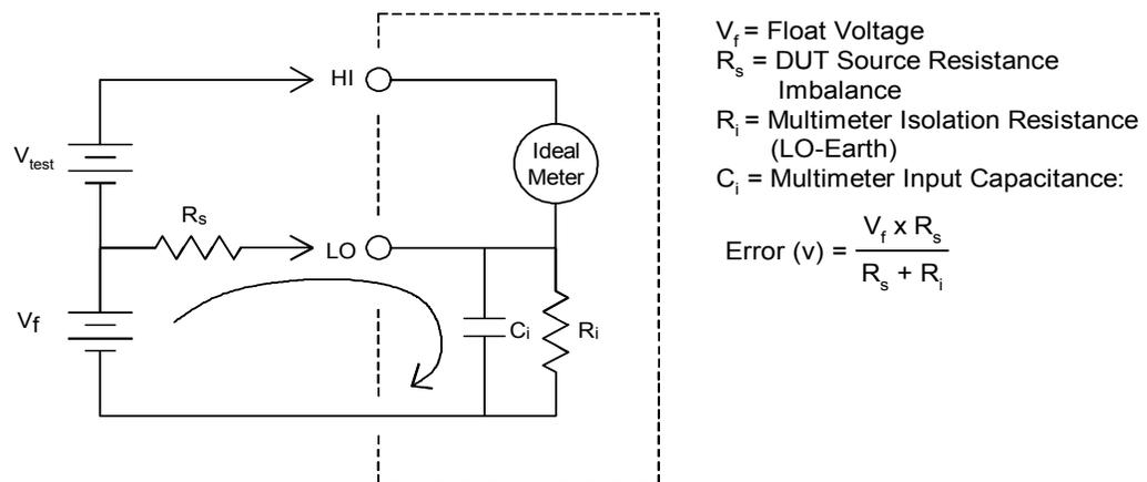
Refer to “[Measurement Noise Rejection](#)” on page 130 for the multimeter’s NMR and CMR characteristics.
