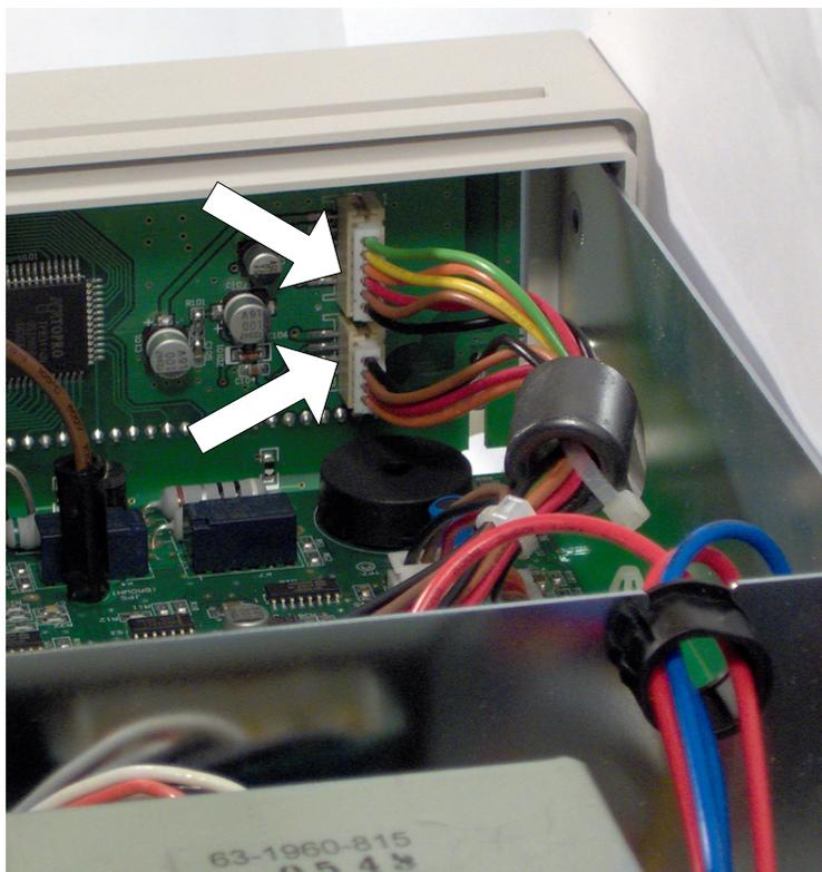
9 Disconnect the individual front panel wires shown below.
