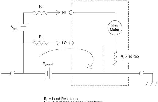
$R_L$  = Lead Resistance  $R_i$  = Multimeter Isolation Resistance  $V_{ground}^i$  = Voltage Drop on Ground Bus
