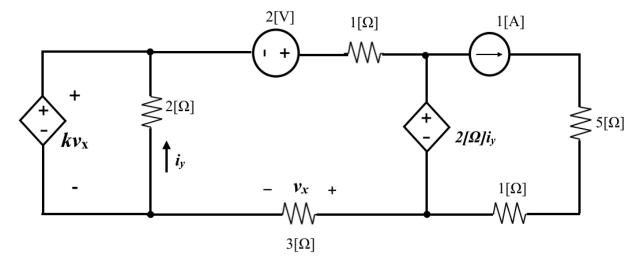
Use the circuit shown below to solve for the numerical values of k and  $v_x$ .
