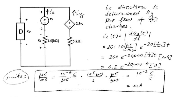
Find  $V_{S}$ (a)  $V_{D} = V_{S} - 1.5 [kn] \cdot ix(t) = 100 [V]$   $V_{S} = 100 + 300 e^{-20,000 t} [V]$   $P_{del}, v_{S} = V_{S} \cdot ix(t)$  $= 20 e^{-20,000 t} + 60 e^{-40,000 t} [W]$
