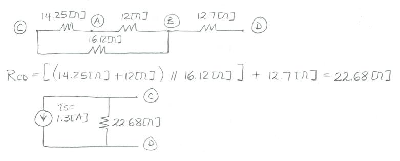
c) Attaching the circuits from a) and b) together, we get:
