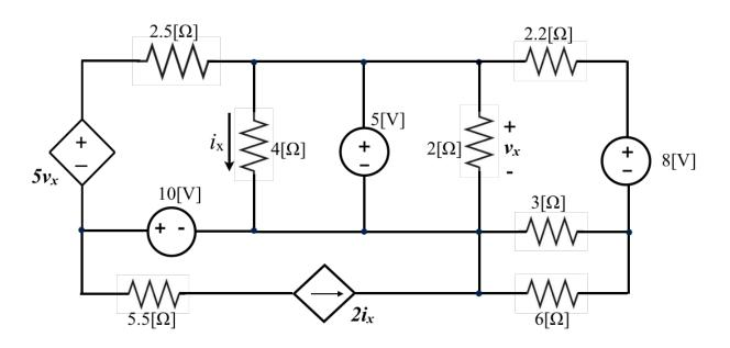
The circuit below has an independent voltage source with a value of 5[V].
