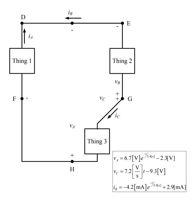
Solution: a) For the power absorbed by Thing 1, we need the voltage across it, and the current through it. The voltage is UA, and the current is LB. The two are in the active sign relationship for Thing 1, so we can write
