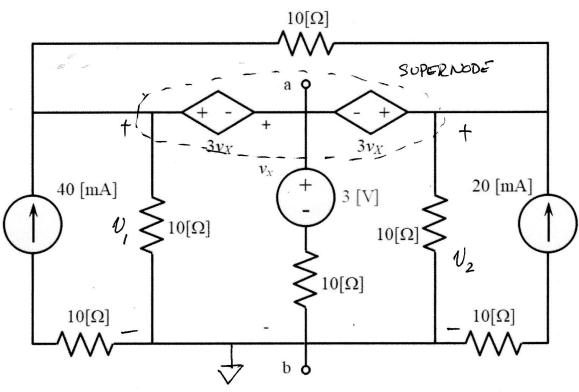
we note that Ux is the open circuit voltage.
