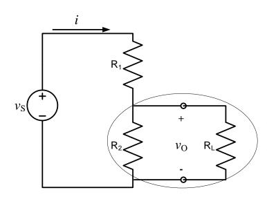
If we add a resistor  $R_L$ , the voltage  $v_O$ will change because the current through  $R_2$  is now different; some of it is being "drawn off" by  $R_L$ . (The current *i* will change, too.) Let's do the calculation...
