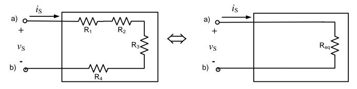
More generally, for 'k' resistors in series, we can define an equivalent given by
