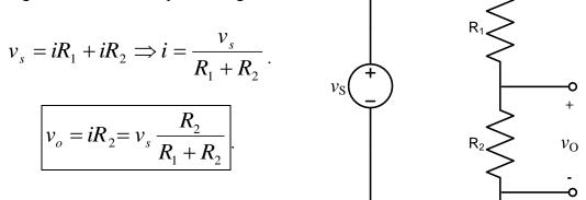
So the source voltage has been "divided" by the two resistors; we have calculated the fraction of the source voltage that appears across  $R_2$ . We could have done a similar thing for  $R_1$ . This is the *voltage divider rule* (VDR).
