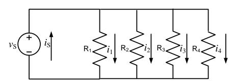
This last equation says that, given  $v_s$ , the current will stay the same if we replace the four resistors with an equivalent  $R_{eq}$ ; that is,
