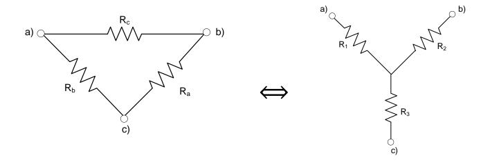
These configurations are interchangeable, but be careful to note the positions of the terminals (a, b, c) relative to the resistors. The formulae for the transformations are...
