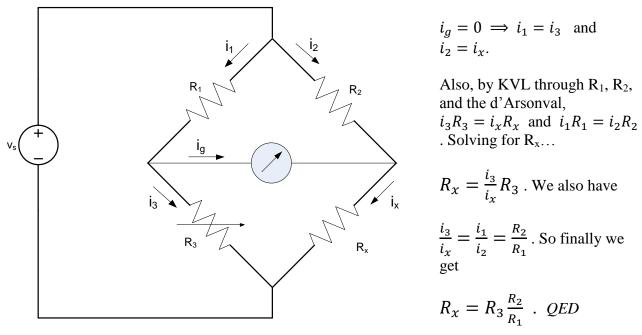
Typically we make  $R_1$  and  $R_2$  adjustable in decades, i.e.,  $R_1$  and  $R_2$  can be set to 1 [ $\Omega$ ], 10 [ $\Omega$ ], 100 [ $\Omega$ ], and 1000 [ $\Omega$ ]. That means  $R_2/R_1 = 0.001, 0.01, ...100, 1000. R_3$  is set to vary from, say, 1 [ $\Omega$ ] to 1000 [ $\Omega$ ] in increments of 1 [ $\Omega$ ]. That will give us a wide range of possible unknown resistances. For practical reasons we should expect to be able to measure
