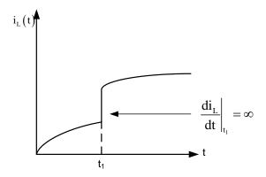
Here, the current changes from one value to another over a time span of 0 [s] at t<sub>1</sub>, i.e., instantaneously. This produces a derivate, and hence a voltage, that is infinity large. We can't have this!!
