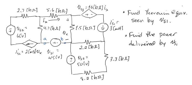
We define terminals a, b, so that we can keep track of polarities. We need two of Noc, isc, Rich via test source. We will do all three. It turns out that is is the longest!
