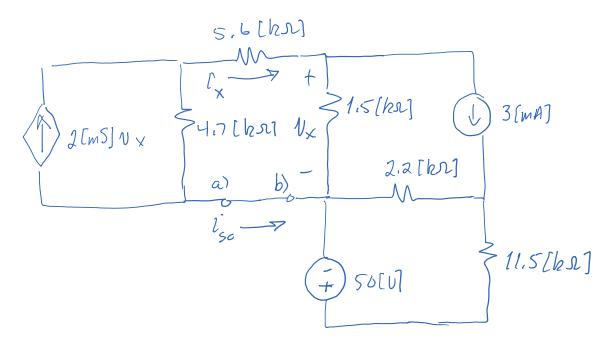
Nothing fancy here, except that I have removed circuit elements in services with the two current sources. Other than that, the mesh current method makes sence because the two current sources mean that two mesh currents are already known. This is clearly the hardest of the three things
