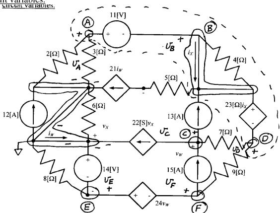
First, using the node-voltage method. We define the node voltages on the diagram above. We will need to write 10 equations (7-1+4).
