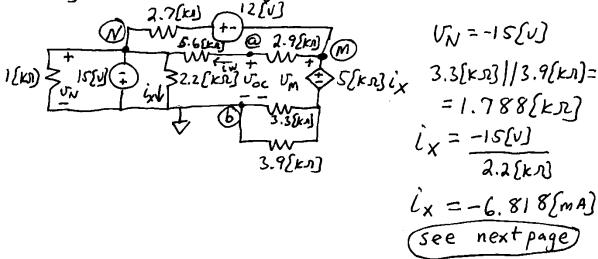
$$\frac{U_{M} + 15[v]}{8.5[kn]} + \frac{U_{M} + 12[v] + 15[v]}{2.7[kn]} + \frac{U_{M} - 5[kn]ix}{1.788[kn]} = 0$$
