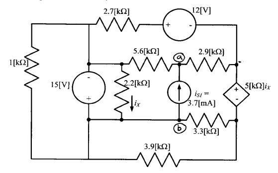
We choose to find Voc. Remove is, and redraw, labelling Voc in the diagram.
