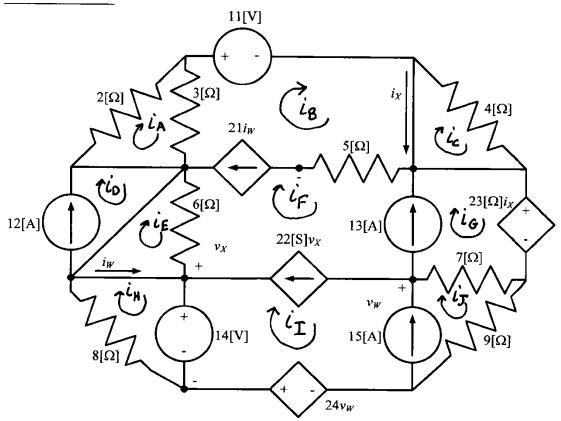
The alternative was to use the mesh-current method. We define the mesh currents on the diagram above. We will need to write 14 equations (10+4).
