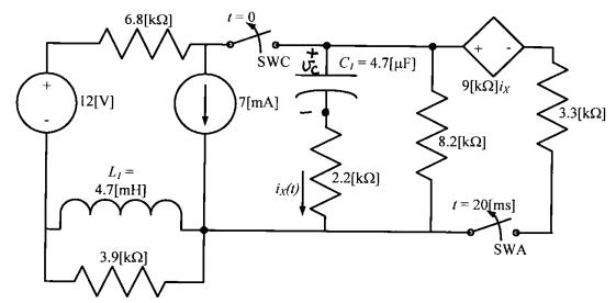
We begin by defining the voltage across the Capacitor C, , which we have done in the diagram above. Then, to get the initial condition, we use the steady-state conditions, and redraw for t<0:/
