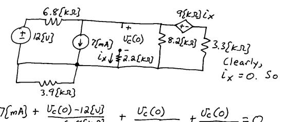
$$7[mA] + \frac{V_{c}(0) - 12[U]}{6.8[KN]} + \frac{V_{c}(0)}{3.3[KN]} + \frac{V_{c}(0)}{8.2[KN]} = 0$$
