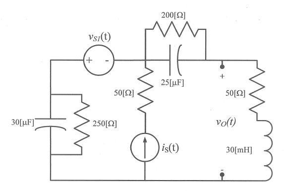
Find the voltage  $v_0(t)$ . The sources are as follows.
