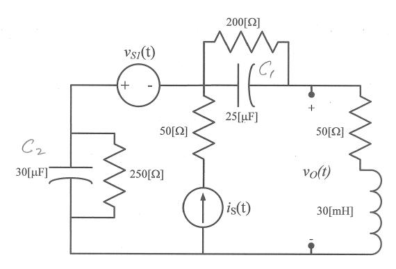
we have sources with two different frequencies: for  $v_{s,1}(t)$ ,  $\omega = 0$  (dc). For  $i_s(t)$ ,  $\omega = 377$  [rad/s], we must therefore use superposition.
