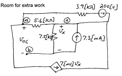
$$\frac{KCL@@)}{5.6[kn]} \frac{V_{OC} - V_{X}}{5.6[kn]} + \frac{V_{OC} + 200[v] - V_{X}}{3.9[kn]} + 7[ms]V_{X} = 0$$
