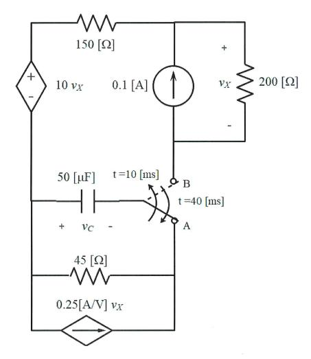
a) we need an initial condition for t<10 lms]: With the switch at A, we have
