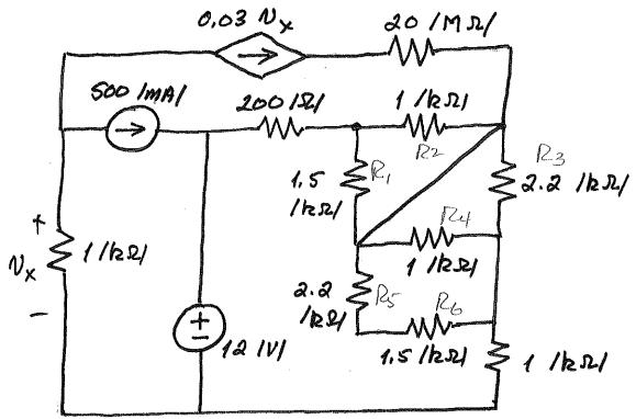
We could attack this problem directly with the node voltage or mesh current method, but it will be easier to reduce the resistor network first,
