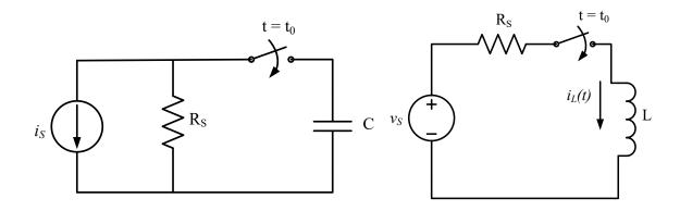
Again, we are using Thevenin and Norton equivalent circuits to represent what gets connected to the inductor and capacitor. Later we will consider more complex circuits.
