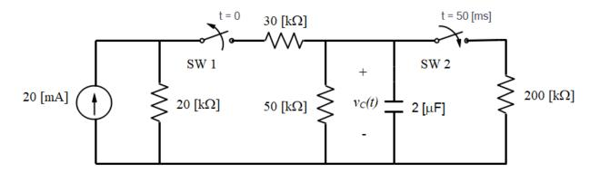
Let's think about what happens here. The circuit below shows what is happening before t = 0. Switch 1 is closed, and switch 2 is open. The current source and resistors create a voltage  $v_C(t_0)$  across the capacitor.
