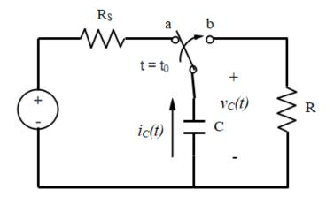
The "natural response" is one in which the capacitor, with a voltage across it, undergoes a switching event that connects it to a resistance only. As for the inductor, that resistance can be a single resistor, or it can be an equivalent resistance that arises from a circuit containing multiple resistors and/or dependent sources.
