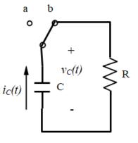
Note that the capacitor current and voltage are in the active sign relationship. You should convince yourself that the signs in this equation are correct. This is a first-order differential equation for  $v_C(t)$ .
