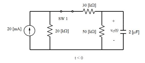
After switch 1 opens, but before switch 2 closes, the capacitor is connected only to the 50  $[k\Omega]$  resistor. This is a natural response problem.
