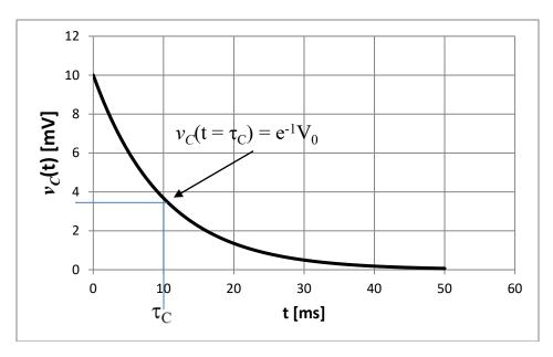
As for the inductor, after five time constants, or t = 50 [ms], the voltage has decayed almost to 0. What is left is less than 1% of the initial value:  $t = 5\tau_C \Rightarrow v_C(t) = 0.0067v_C(t_0)$ . As we pointed out above, we define a "long time" as five time constants.
