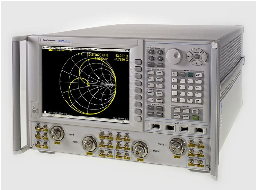
A network analyzer (Agilent N5245A PNA-X) showing a Smith chart.
