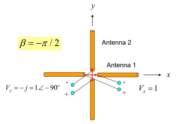
This antenna will radiate a RHCP signal in the positive z direction, and LHCP in the negative z direction.
