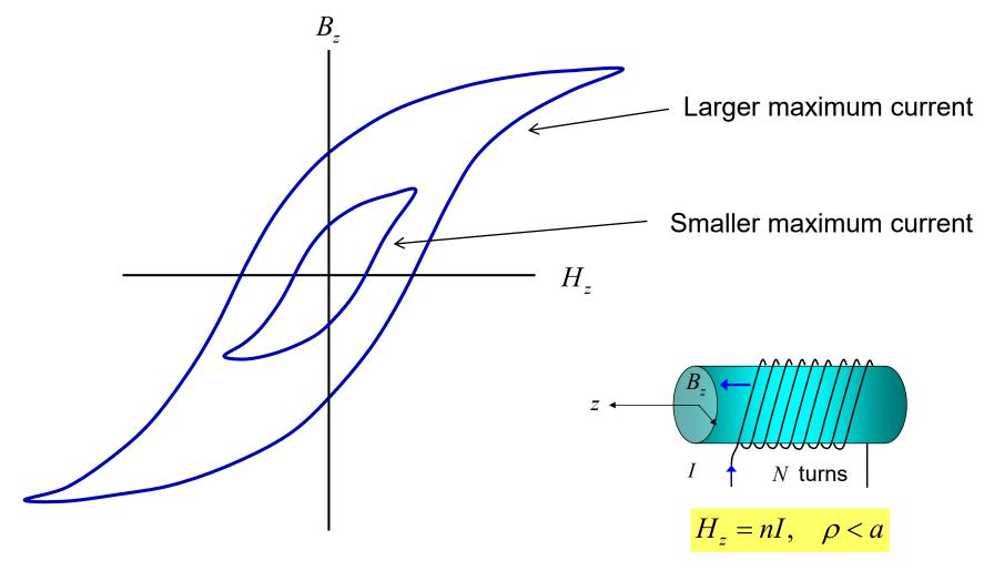
Hysteresis causes <u>power loss</u> for an AC magnetic field in a nonlinear material (such as in a transformer core).
