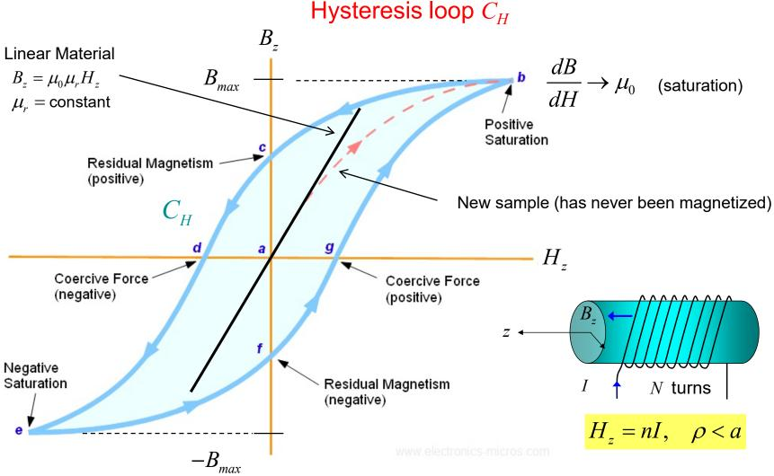
Note: The size of the hysteresis loop depends on the maximum current in the coil.
