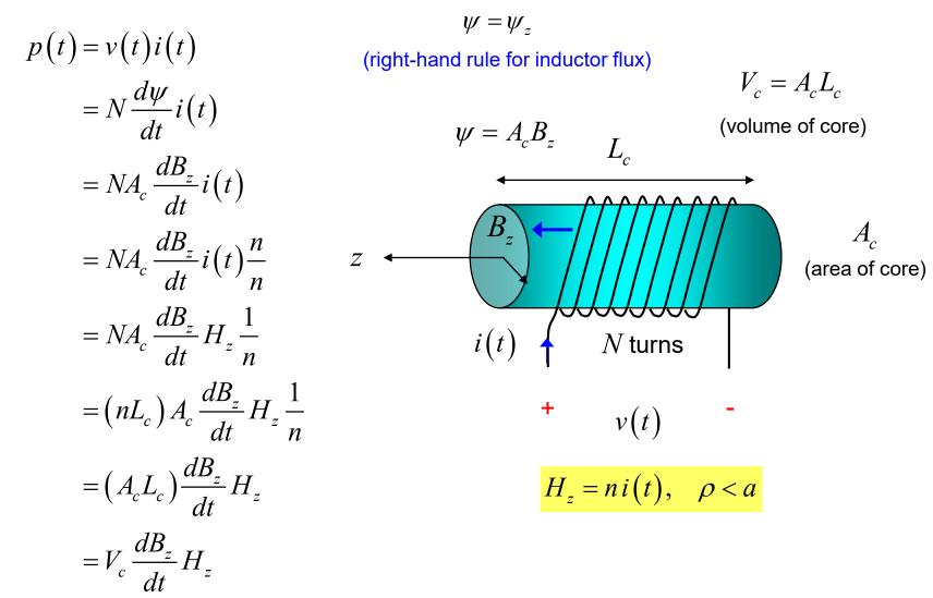
Energy going into the coil in <u>one cycle</u> of the waveform (period *T*):
