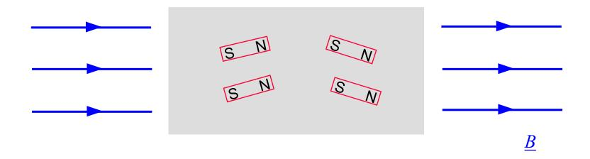
Because of *electron spin*, atoms tend to acts as little current loops, and hence as electromagnetics, or bar magnets.
