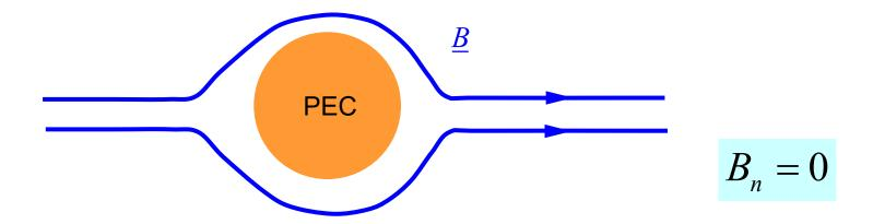
Magnetic field lines must bend around a perfect electric conductor (PEC). This is the opposite behavior of electric field lines.
