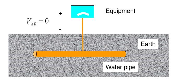
Physical grounding is usually to underground pipes and conductors.
