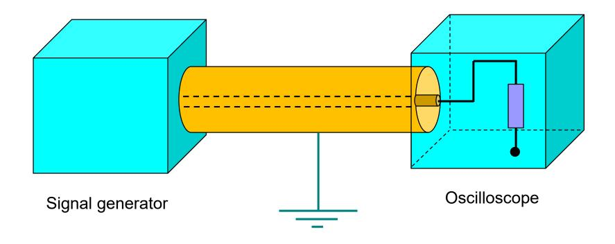
The outer conductor "shield" of the coax is grounded because it is connected to the metal chassis of the equipment, and this is grounded (via a three-prong plug).
