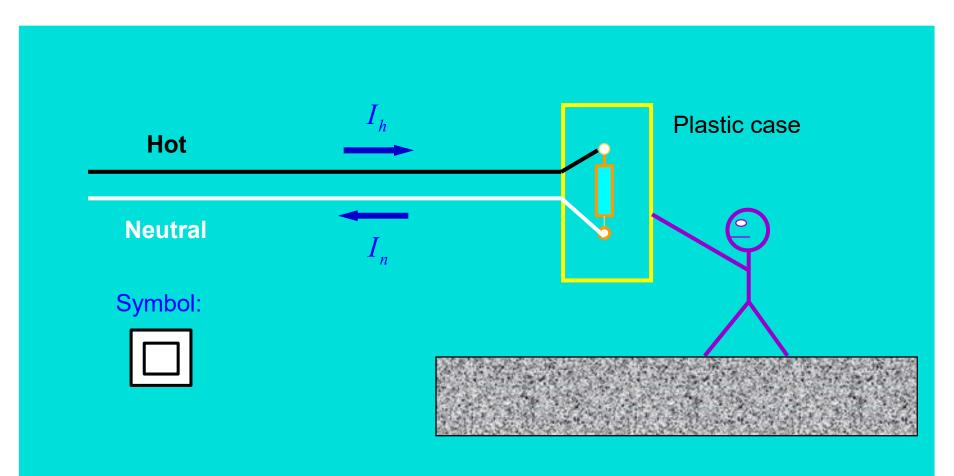
The device has two layers of insulation (usually the case is an insulating plastic case). It does not require a ground.
