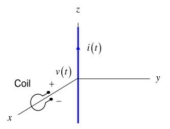
9) A coil of wire has N = 1000 turns (loops). The area of each loop is 100 [cm<sup>2</sup>]. The total length of the wire in the coil has a resistance of 10 [ $\Omega$ ]. The loops lie in the z = 0 plane (see the figure below). A 60 [Hz] magnetic field is applied to the coil, having the form
