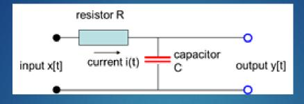
Q.4 For all time t<0, input x[t]=1 Volt. Suddenly at t=0, the input is switched to 0 V (with zero impedance at the input). Sketch your best guess what voltage y[t] looks like as a function of time for t>=0. Extra credit if you write the correct mathematical expression for y[t].
