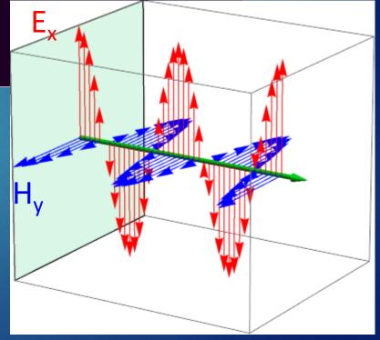
Finite-Difference Time-Domain (FDTD) method is a powerful algorithm to solve Maxwell's equations numerically for problems with complex geometry and media (brute force approach).
