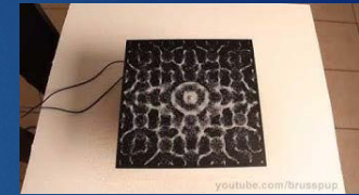
Chladni Plates Harvard Natural Sciences Lecture Demonstrations Four centrally mounted brass plates are driven into resonance. The patterns that appear on the plates help ...
