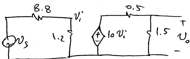
c)  $R_i = 1.2 \text{ k}\Omega \quad R_o = 0.5 \text{ k}\Omega$
