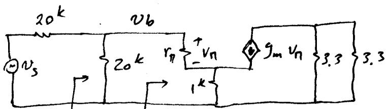
d)  $R_i^! = r_n + 1(101) = 103 \text{ k}\Omega$
