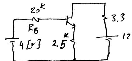
b)  $r_n = \frac{\beta V_T}{I_C} = \frac{100 \times 25}{1.22} = 2.049 [\text{k}\Omega] \quad g_m = \frac{I_C}{V_T} = \frac{1.22}{25} = 48 \text{ mV}$
