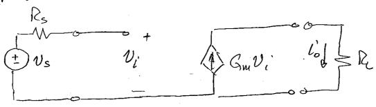
$$\int G_{11} = \frac{l_{0}}{v_{i}} = \frac{l_{0}}{v_{s}} = \frac{-Av_{0}Ai}{2R_{0}+R_{i}} = \frac{-25\cdot(0.15)}{2k+4.9k} = -5.6\times10^{-4} P_{V}$$
