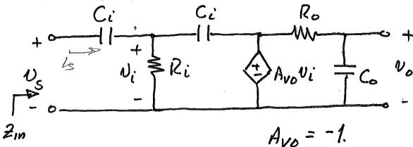
$$\frac{\overline{V_i}}{R_i} + \frac{\overline{V_i - V_s}}{|J_j w C_i|} + \frac{\overline{V_i - A_{vo} V_i}}{|J_j w C_i|} = 0$$
