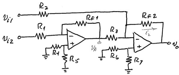
$$V_{A} = -\frac{R_{F}}{R_{A}} V_{i2}$$
