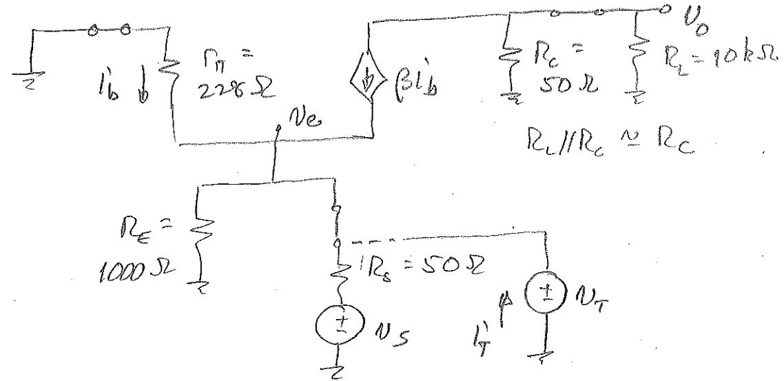
a) Replace  $V_s$ ,  $R_s$  with a test voltage. Then
