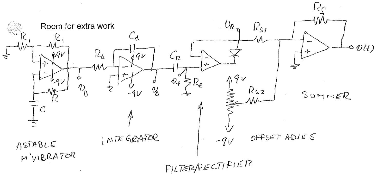
Astable mv:  $T = 2RC \ln \frac{1+\beta}{1-\beta}$        $R_1 = 10k\Omega \Rightarrow \beta = \frac{R_2}{R_1+R_2} = 0.5$
