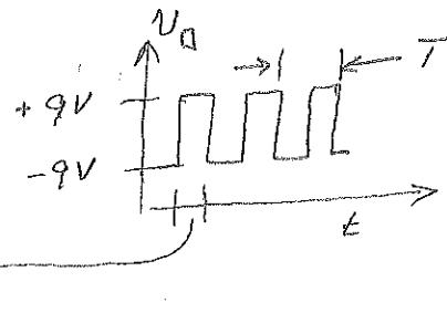
Integrator:  $V_A = -\frac{1}{R_A C_A} \int_0^{T/2} V_B dt = -\frac{1}{R_A C_A} 9 \cdot \frac{T}{2} = -4 \text{ V}$
