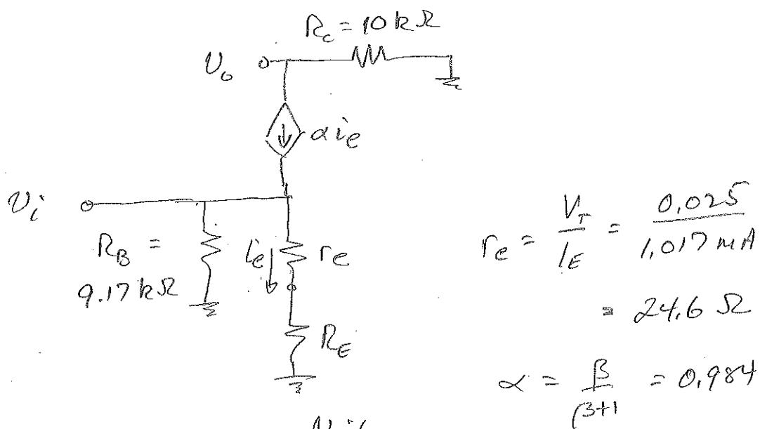
$$V_o = -\alpha i_e R_C \quad i_e = \frac{V_i}{(r_e + R_E)}$$
