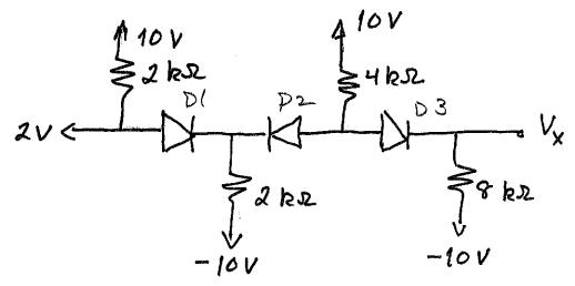
The -10 V sources and the 10 V sources are in a position to forward bias all diodes. Let's try that:
