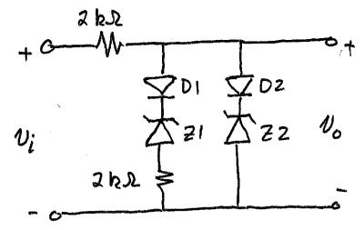
a) To have DI and 21 conducting, we used  $V_0 > V_{4h} + V_2 = 0.6 + 2.4 = 3.0 V$
