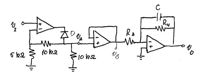
a) The first stage is a "superduce". With the ducto polarity indicated, D will be on when 1/2 to and off when 1/2 to. So NA is a negative going harf wave,
