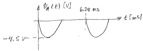
The gain is  $\frac{V_{4}}{V_{2}} = 1 + \frac{10 \, h \, R}{5 \, k \, J \, L} = 3$ , so  $V_{4, \text{max}} = -4.5 \, V$ .
