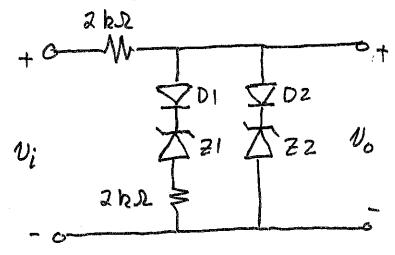
3. (35 points) The diodes in the circuit below are modeled with  $V_{th}$  = 1 V,  $r_d$  = 1 k $\Omega$ , and  $I_S$  = 1 mA. Find  $V_X$ .
