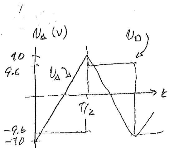
$$\text{choose } C = 0.1 \mu\text{F} \Rightarrow R_V = \frac{9.6 T}{2} \frac{1}{20} \frac{1}{0.1 \times 10^{-6}} = 2.4 \times 10^6 \Omega$$
