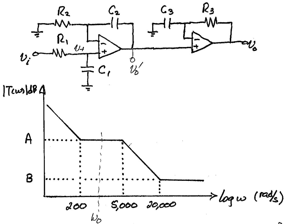
a) Define  $\bar{V}_+$ . Then  $\bar{V}'_o = \bar{V}_+ \left(1 + \frac{j\omega C_2}{R_2}\right) = \bar{V}_+ \left(\frac{1+j\omega C_2 R_2}{j\omega C_2 R_2}\right)$
