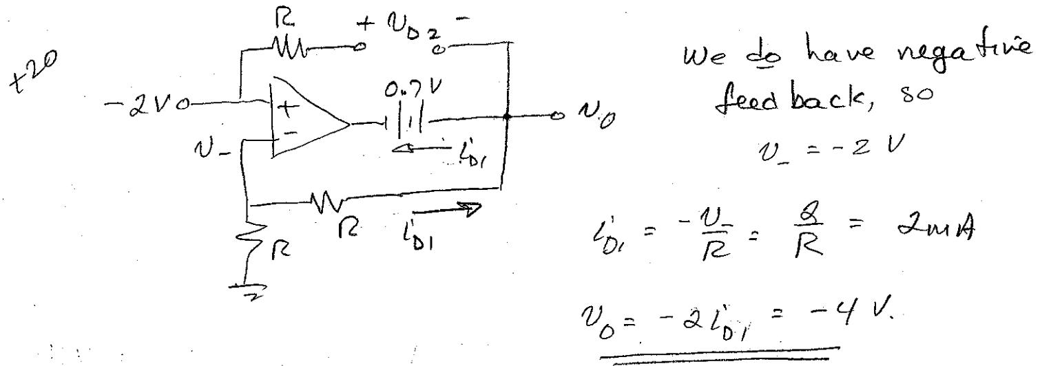
Diode check:  $i_{D_1} = 2 \text{ mA} \checkmark$
