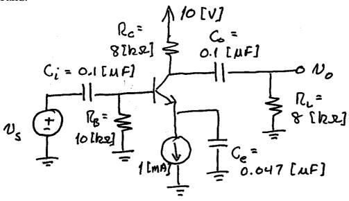
In the passband, all capacitors are shorted. If they are open-circuit, then either the upit would be cut of (Ci), the output would be cut of (Co), or the confler would be open-circuit to ac (Ce),
