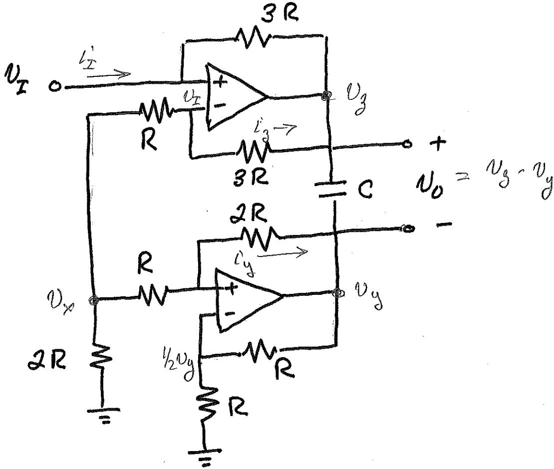
Node voltage at  $v_x$ :  $\frac{v_x}{2R} + \frac{v_x - v_i}{R} + \frac{v_x - \frac{1}{2}v_y}{R} = 0 \quad (1)$
