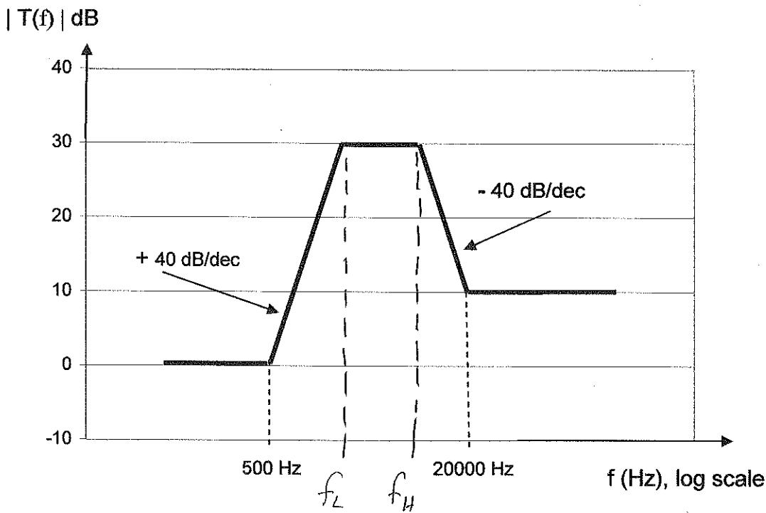
We need to identify  $f_L$  and  $f_H$ . We note that at  $f_H$ ,  $T(f)$  has increased by 30 dB at a rate of 40 dB/dec - this requires  $\frac{30}{40} = 0.75$  decade. Also,  $f_H$  to 20000 Hz requires  $\frac{20 \text{ dB}}{40 \text{ dB/dec}} = 0.5$  decade.
