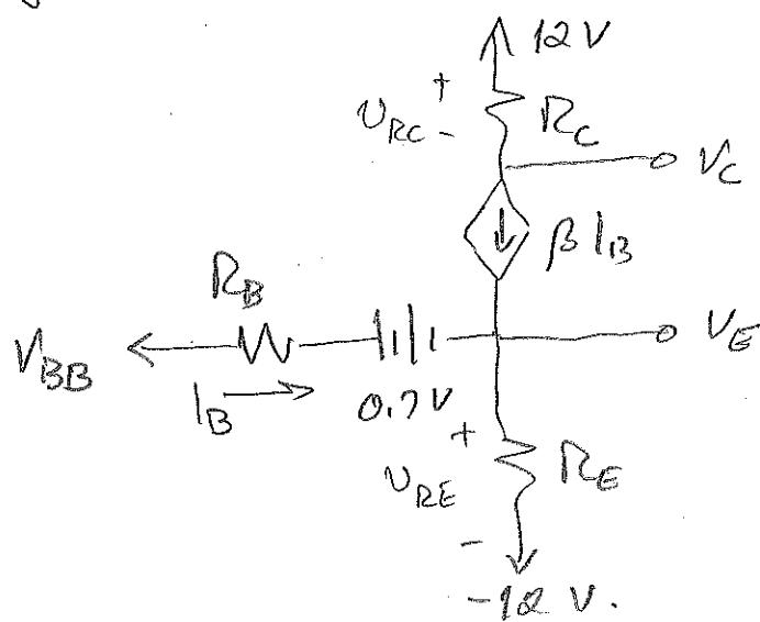
We can choose  $V_{BB} = 0$ , which makes  $R_{B1} = R_{B2}$ .
