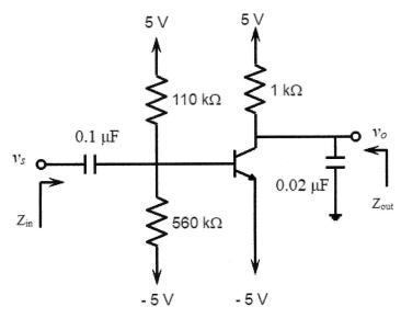
we will use the hybrid-pi model so we'll need Therenin equivalent at the base:  $V_{BB} = 10 \frac{560}{560+110} - 5 = 3.36V$
