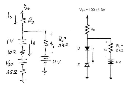
The diode models are inserted into the circuit in the figure above.
