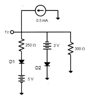
2. (33 1/3 points) For the circuit below, the diodes are modeled using a piece-wise linear model with  $V_{th}$  = 1.0 V,  $r_D$  = 5  $\Omega$ , and  $I_S$  = 0.
