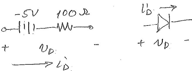
{ Extrapolating the  $I_D$ - $V_D$  curve to the  $I_D=0$  axis  $\Rightarrow$  Voltage source is -5 V. Taking the inverse of the slope  $\Rightarrow$  resistance is  $\frac{\Delta V}{\Delta I} = \frac{1V}{10mA} = 100\Omega$ .
