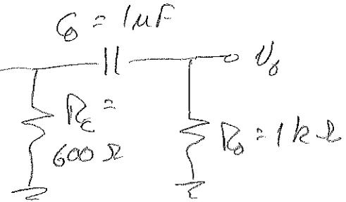
$$\bar{V}_o = -\beta \bar{I}_b \cdot \frac{R_o}{j\omega C_o + R_o + R_C} R_o = -\beta \bar{I}_b \cdot \frac{j\omega C_o R_o \cdot R_C}{1 + j\omega C_o (R_o + R_C)}$$
