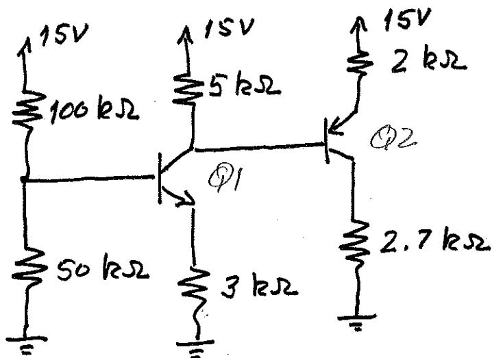
We will guess linear region for both. Given  $15V$  and  $0$  as shown, we expect current to be flowing top to bottom, which is linear region for both BJTs.
