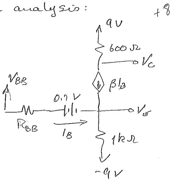
$$I_B = \frac{3.6 + 9 - 0.7}{21000 + 101(1000)} = 97.54 \mu A \quad \checkmark$$
