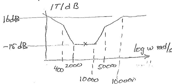
In principle, knowing  $|T(\omega=4500 \text{ rad/s})|$  and all slopes, we do not need to know K. We will solve for it anyway...
