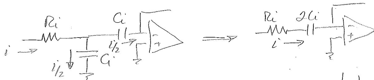
This correctly predicts the input impedance but it does not give the correct output. For that we need a more complete analysis. Looking at the original circuit:
