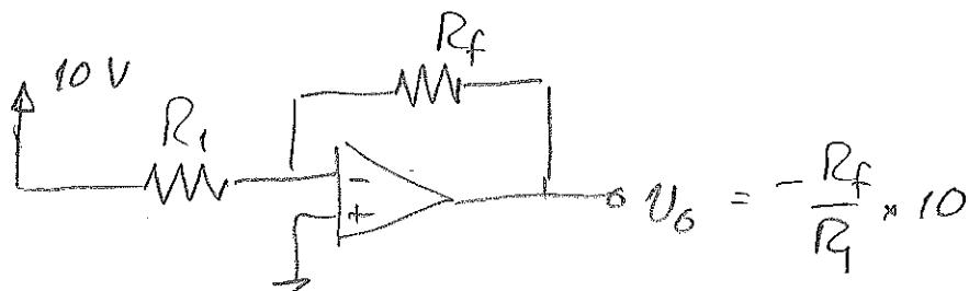
In this case, we need  $v_o = -4 \text{ V}$ ,  $\Rightarrow \frac{R_f}{R_1} = 0.4$
