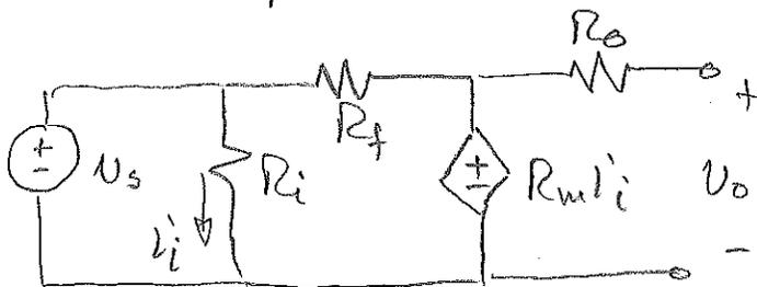
$$v_o = R_m i_i = R_m \frac{v_s}{R_i}$$
