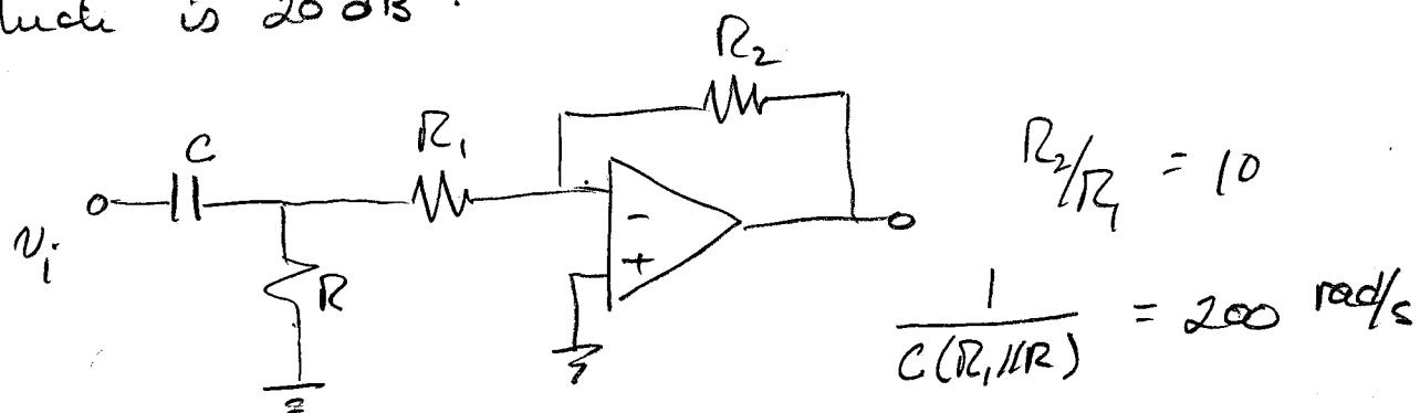
If we want to isolate the filter first, we can use a buffer amp:
