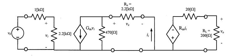
Two amplifiers are cascaded as shown, with a resistor  $R_x$  connecting the two. A source  $v_s$  and load  $R_L$  are also shown. The source resistance is 0. The gain parameters  $G_m$  and  $R_m$  are not specified, but it is known that when  $v_s = 10$  mV,  $v_x = -8.653$  V and  $v_o = -893.86$  mV.
