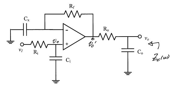
$$V_{0}' = V_{+} (1 + \int w C_{x} R_{f})$$
