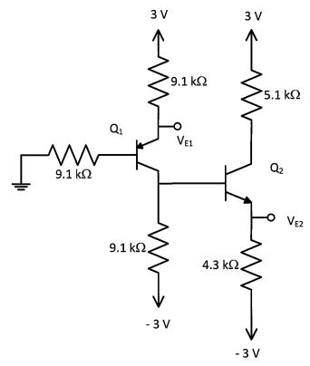
Looking at the flow of charge carriers, it seems clear that holes will move from Q1 emitter into Q1 base and then out through the collector, Same for electrons in Q2, So we assume active region for both.
