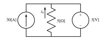
2. Find the Thévenin equivalent resistance seen at terminals a and b in the circuit below.
