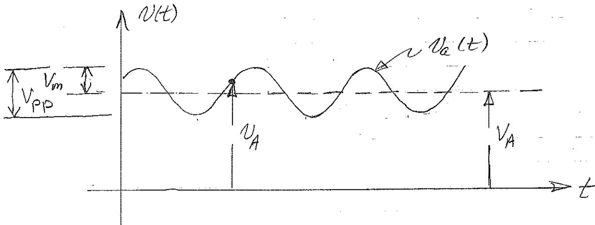
AC COMPONENT:  $V_a(t) = V_m \sin(\omega t + \phi)$
