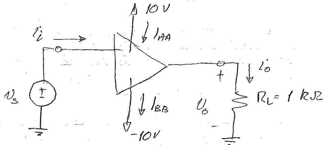
Given:  $I_{AH} = 1 \text{ mA}$     $I_{BB} = 0.5 \text{ mA}$
