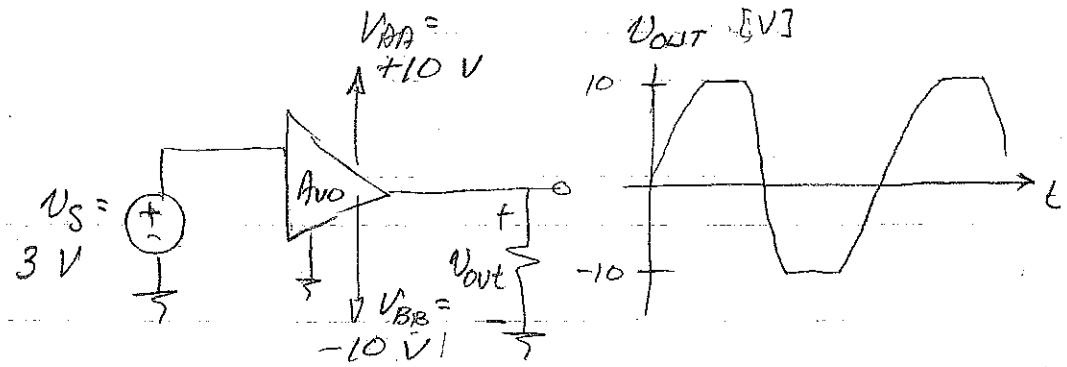
Suppose  $A_{v0} = 5 \Rightarrow V_o = \pm 15V$  ! This will be clipped to  $\pm 10V$ .
