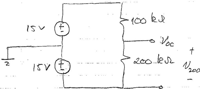
$$V_{200} = (30\text{ V}) \cdot \frac{200\text{ k}}{200\text{ k} + 100\text{ k}}$$
