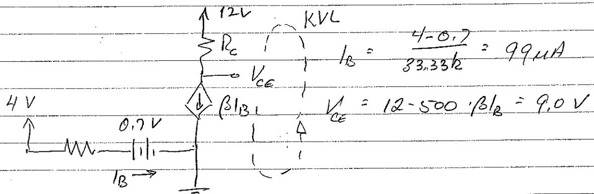
We can now go to the  $I_C$ - $V_{CE}$  plot and locate our Q-point. It is at  $I_B = 99 \mu\text{A}$  and  $V_{CE} = 9.0 \text{V}$ .
