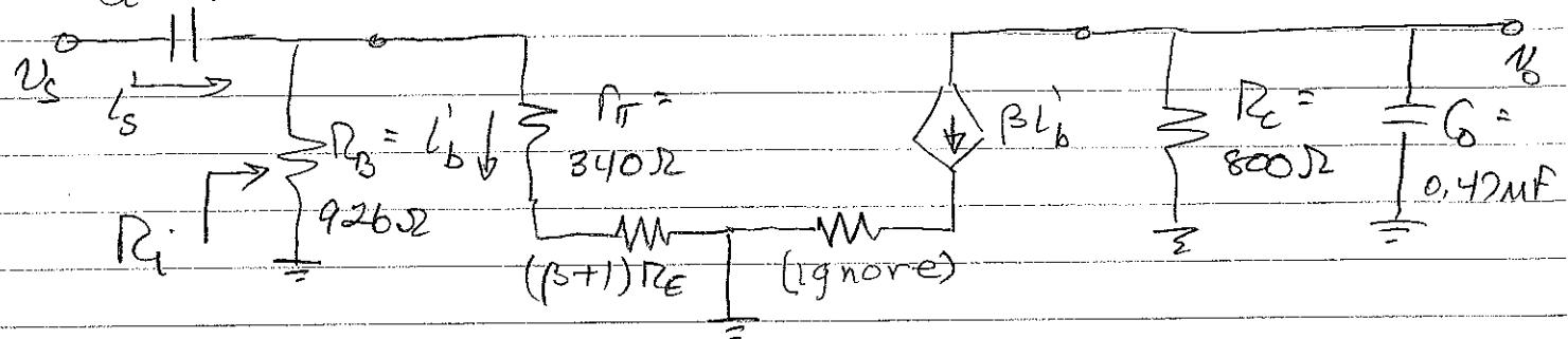
Let's simplify the input a bit. The resistance  $R_i$  is
