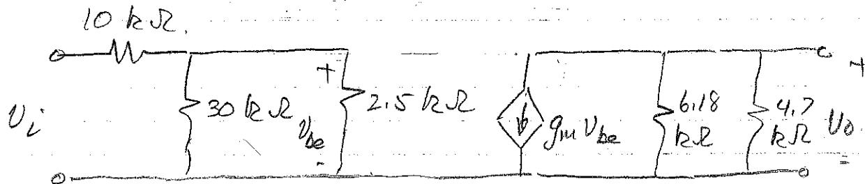
$$\frac{V_{be}}{V_i} = \frac{2.5k/130k}{2.5k/130k + 10k} = 0.187$$
