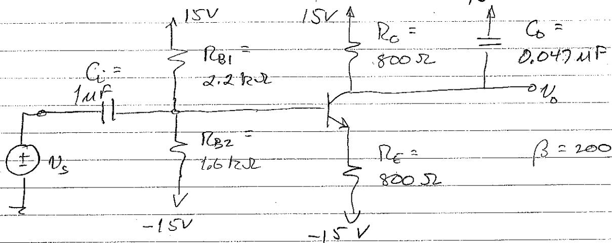
This is a small-signal analysis problem, but we need a dc analysis to find the necessary ac model parameters. We should also check to be sure we are biased in the linear region.
