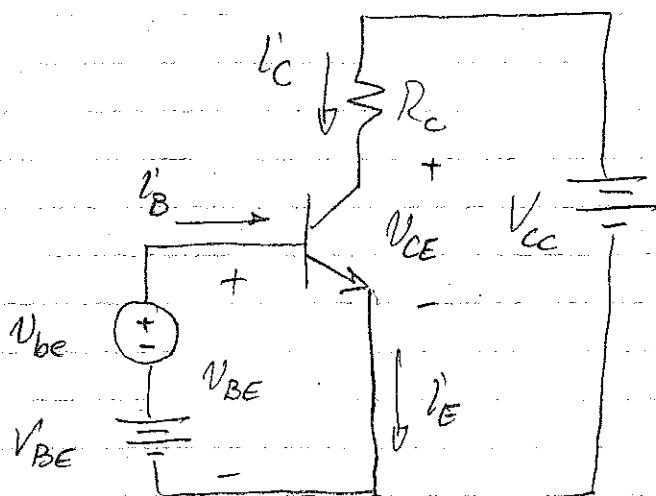
$$I_C = I_S e^{\frac{V_{BE}}{V_T}} \quad (V_{BE} \gg V_T)$$
