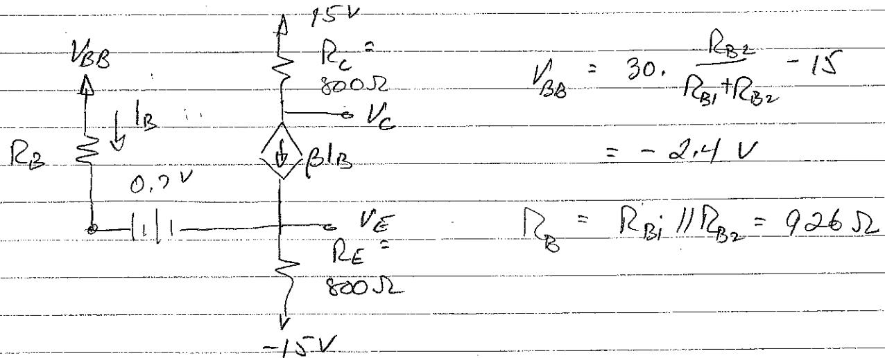
$$KVL: -V_{BB}'' + R_B I_B + 0.7 + (\beta+1) R_E - 15 = 0$$
