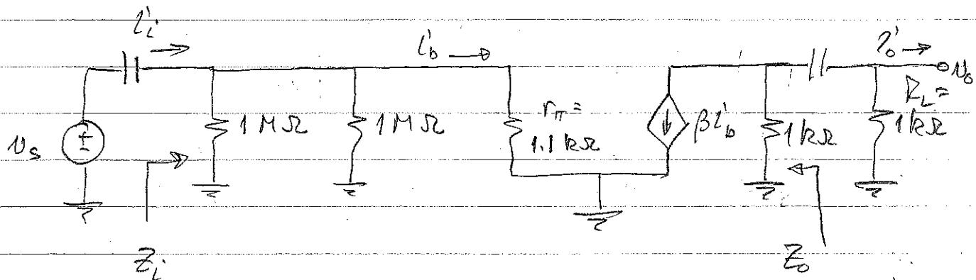
$$r_\pi = \frac{V_T}{I_B} = \frac{25mV}{22.6\mu A} = 1.1k\Omega$$
