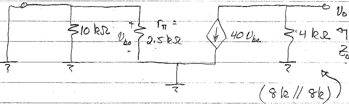
$$\text{Now } V_{be} = 0 \Rightarrow 40 V_{be} = 0 \Rightarrow \underline{\underline{Z_o = 4 k\Omega}}$$
