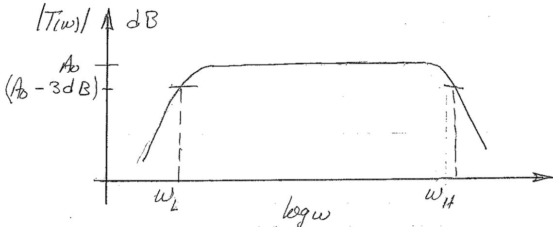
The frequency range over which the gain is approximately constant is called the **PASSBAND**.
