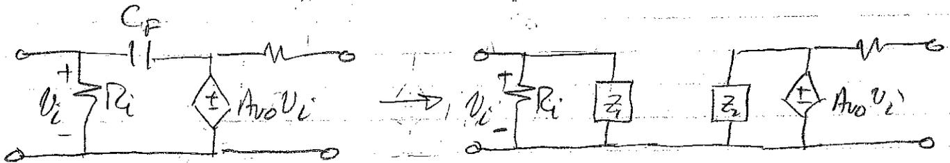
Here,  $Z \equiv 1/j\omega C_F$  and  $K = \frac{A_{vo} V_i}{V_i} = A_{vo}$
