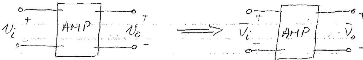
$$T(j\omega) = \frac{\bar{V}_o}{\bar{V}_i} = \underbrace{\left| \frac{\bar{V}_o}{\bar{V}_i} \right|}_{\text{magnitude}} \underbrace{\angle \frac{\bar{V}_o}{\bar{V}_i}}_{\text{phase}}$$
