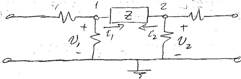
Suppose a circuit has a segment such as that above, where an arbitrary impedance  $Z$  is connected between nodes 1 and 2.
