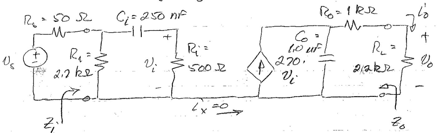
$Z_i$ : Since  $i_x = 0$ , the right-hand side of the circuit has no effect on  $Z_i$ . So...
