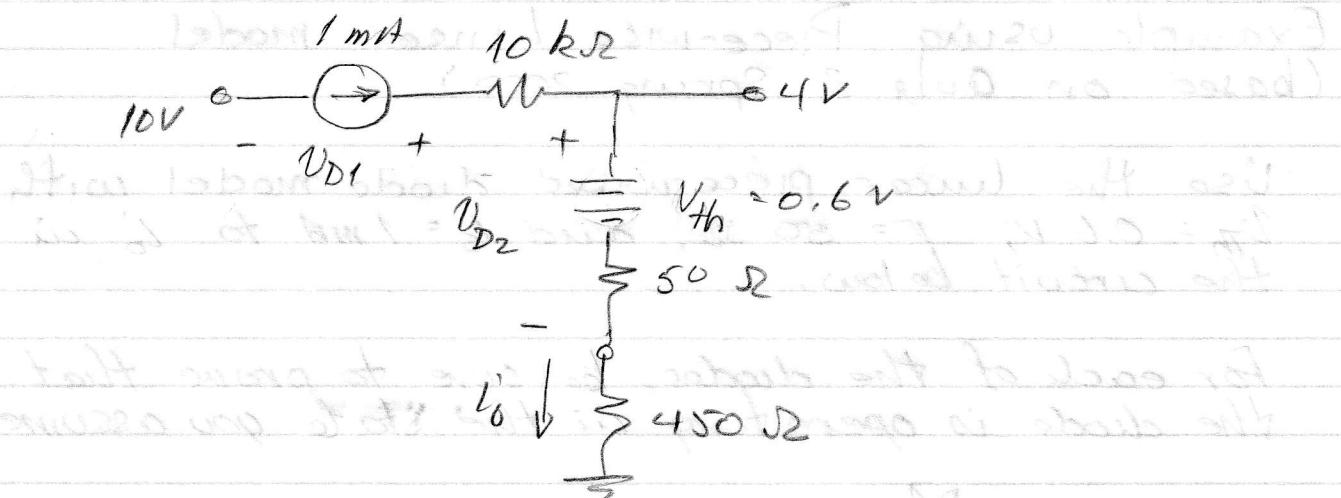
NOTE the polarity of  $V_{D_1}$ . The current source is positive as shown. Note also that  $V_{D_2}$  includes both  $V_{Th}$  and the voltage across  $R$ .
