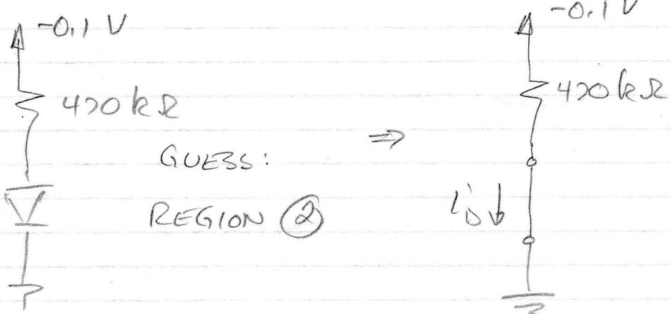
TEST:  $0 \geq i_D \geq -1.0 \times 10^{-6} \text{ A}?$
