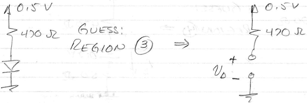
The power supply (0.5V) is positive but not sufficient to turn the device on, so we guess region ②.
